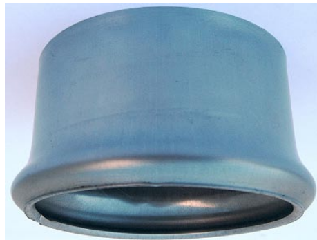
Figure 6: Experimental result showing buckling initiation at the bottom of cup wall.
