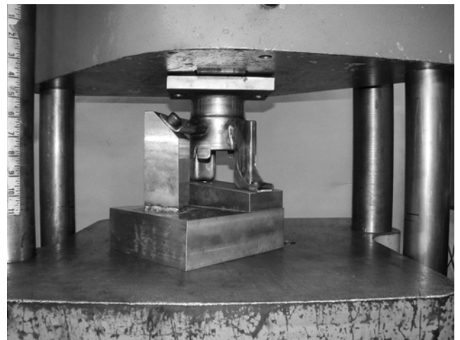
Figure 8: Test setup for static compression testing shown with TC4 product configuration.
