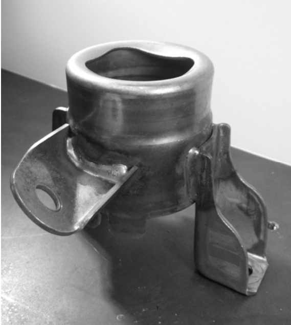
Figure 9: Baseline test configuration sample showing buckling on the top of the can.
