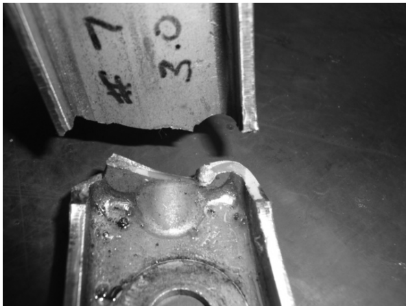
Figure 13: Failure mode after 232,745 cycles with TC2 specimen made from AHSS steel.
