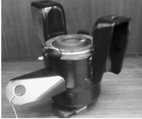
Figure 2: Current hydro-mount assembly with the inner mount press fit into the outer bracket.
