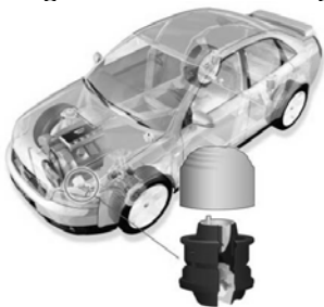
Figure 1: Typical hydro-mount shown in vehicle position ( http://www.trelleborg.com )
